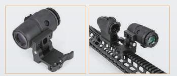
To use the included flip mount, simply apply direct pressure and flip the Magnifier to the left or right side (depending on mounting direction). To return, simply push magnifier back into original position.
